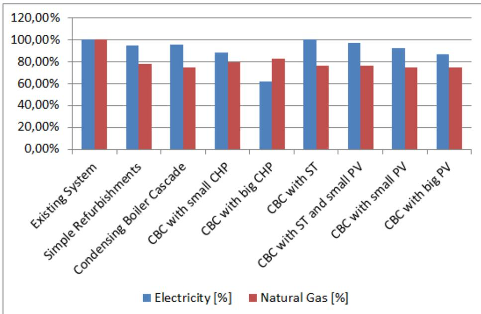
Figure 3: Simulation results for different system variants of school complex
