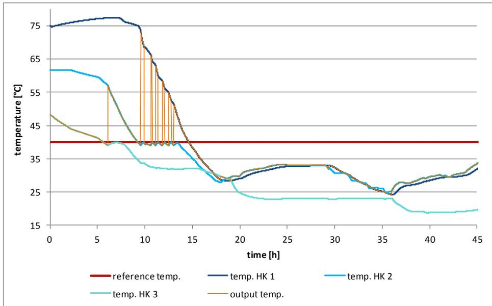
Figure 3: function of the temperature switching valve
