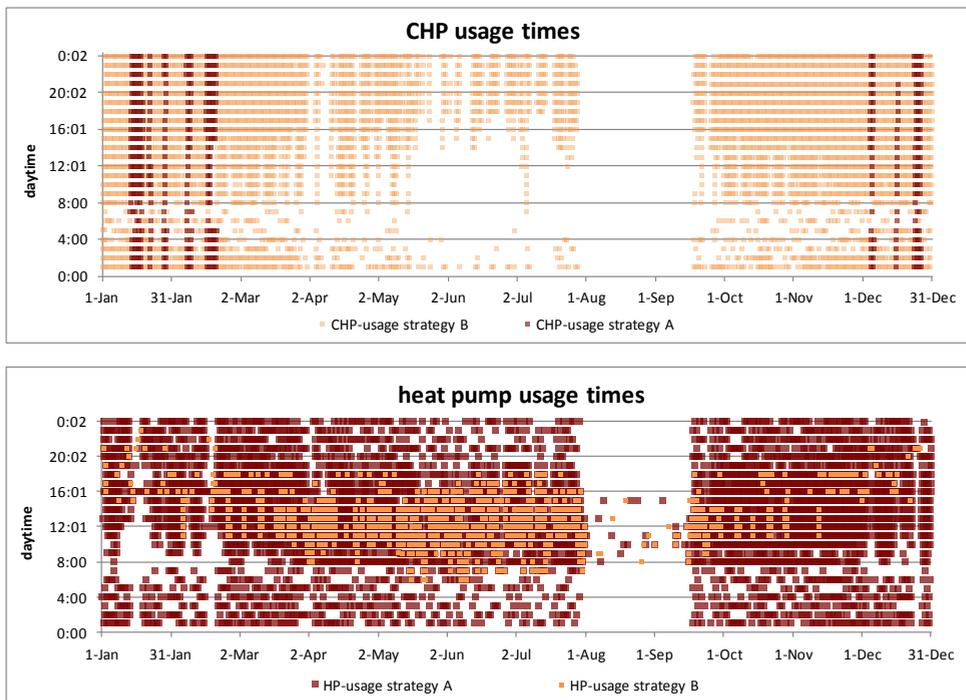
Figure 4: Visualization is important to easily interpret results; usage of CHP (top) and heat pump (bottom) for domestic water supply depending on operational strategy: A - dark, B - light [3]
