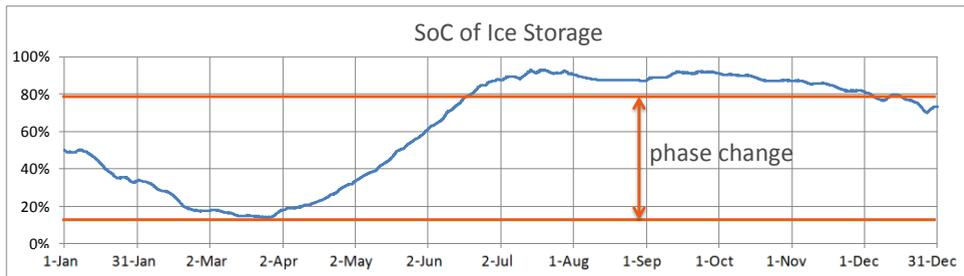
Figure 5: typical 'state of charge' of ice storage with melting heat
