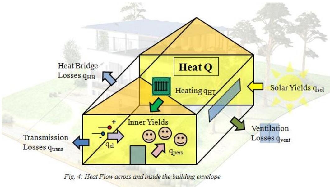
Fig. 4: Heat Flow across and inside the building envelope
