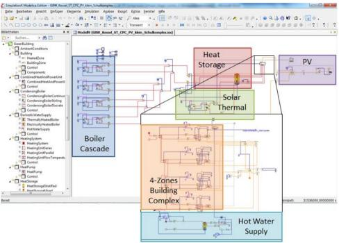
Figure 2: Model of school complex with 4 thermal zones hot water supply as well as energy supply by a boiler cascade, a photovoltaic and solar thermal system
