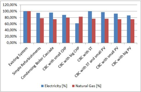
Figure 3: Simulation results for different system variants of school complex
