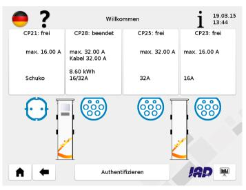
Fig. 4. Screenshot of the user interface (E-City-Routing charging station) as seen on the local touchscreen or in remote administration
